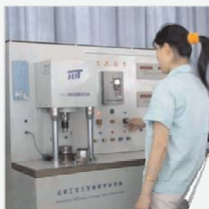
HDM10端面摩擦磨损试验机 HDM10 End-face Friction & Wear Experiment
